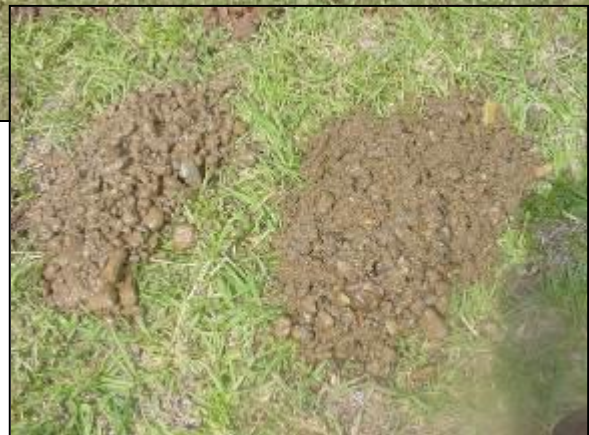
Samples of the materials taken from the bore hole at approximately 1m intervals during drilling. Note high gravel content at depths >10m
